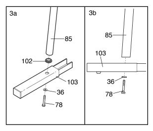
Slide the upper end of a Handrail (85) and then the Extension Leg (103) into the right Upright (82) as shown. (Note: It may be helpful to tip the Uprights [82] forward as you insert the Extension Leg.)
